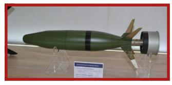
APR 155 weighs around 45 kilograms, its maximum range exceeds 20 kilometres. It remains able to attack targets with accuracy brought down to a couple of meters, this applies to targets that are both moving and stationary. The primary variant of the APR 155 round would feature a HE charge.
