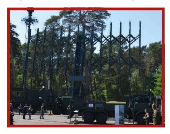
P-18PL radar name is derived from the Soviet P-18 design operated in the meter band frequency range. The radar has been made out of new elements in its entirety, and the bandwidth was broadened. An entirely new VHF AESA antenna array is the main distinguishing element of the system, with an electronically controlled and shaped beam and control of the antenna receiving array in azimuth (despite the
